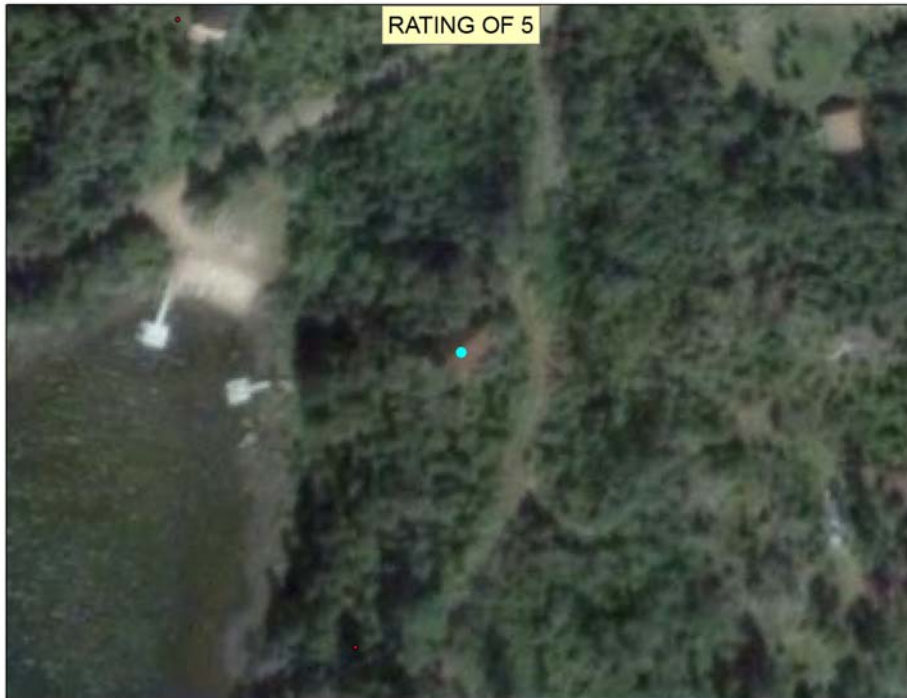
Figure A-6. Example of House Rating No. 5: This building is completely enclosed by trees on all four sides. (source: Google Earth Imagery Digital Media. Available online at http://earth.google.com . Accessed 5/30/08.)
