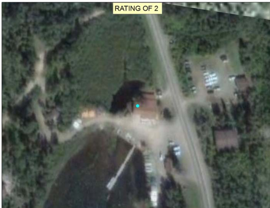
Figure A-3. Example of House Rating No. 2: This building is clearly out in the open; there are trees in the general vicinity but nothing within a house length. (source: Google Earth Imagery Digital Media. Available online at http://earth.google.com . Accessed 5/30/08.)
