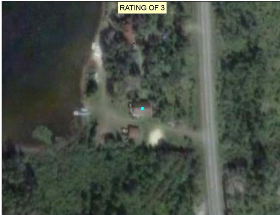
Figure A-4. Example of House Rating No. 3: This building is generally in a clearing, but there are trees on the north side that are within 1 house length. (source: Google Earth Imagery Digital Media. Available online at http://earth.google.com . Accessed 5/30/08.)
